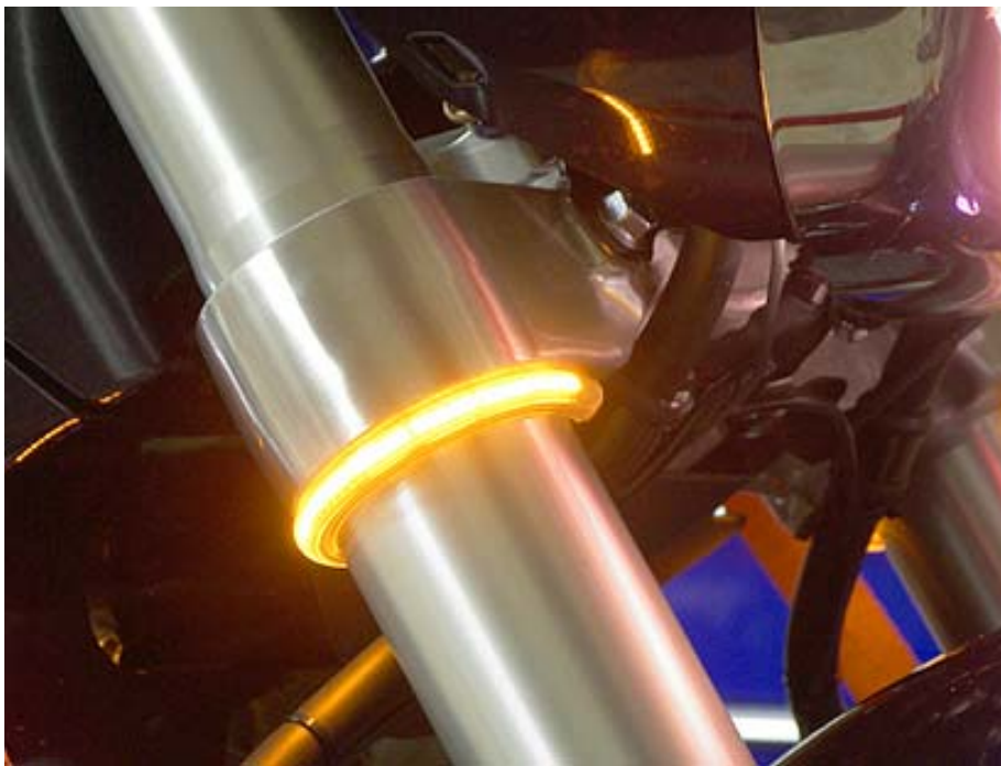
Amber 40 LED Array used as front blinker on a Suzuki M109R
